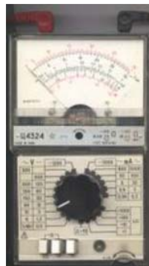
fig.2 analogue multimeter
